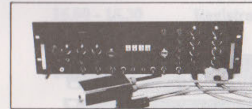
TEC-01C Double Electrode Clamp System for Oocyte Research with Capacitive Transient Compensation
